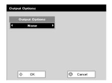
If **None** in the **Output Options** is selected it is only possible to print with the built-in printer or save the data on a connected USB flash drive. No data transfer to a PC is possible. To transfer the data on the result screen to a PC press 9 for **Output Options**, change the **Output Options** to the device of choice.
