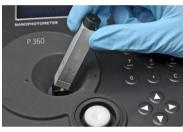
Insert the NanoPhotometer® P-Class Submicroliter Cell into the cell holder with the cell windows facing the light beam. We recommend facing the Implen logo to the front. The light beam is directed from RIGHT to LEFT as indicated with small arrows. Insert the NanoPhotometer® P-Class Submicroliter Cell always in the same direction.
