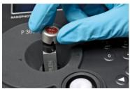
Make sure that for the measurements the lid fits exactly onto the positioning supports mounted to the body of the cell. Take measurement. **Remember** to consider the lid factor in your instrument software. Please refer to the NanoPhotometer® P-Class User Manual for detailed information.
