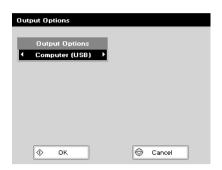
Select how the data are send. Options are *Computer (USB)* or *None*. Press *OK*to store the settings and return to the *Utilities* folder *OR* press *Cancel* to return to the *Utilities* folder without storing the settings.
