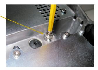
Figure 86 Instrument inlet purge port securing bolt
