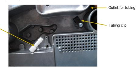
5. Locate the sample compartment purge connector shown in Figure 85.
