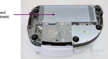
Figure 91 Location of the main board compartment
