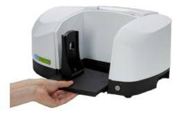
Figure 25 Removing the sampling accessory
