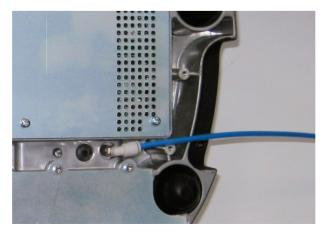
Figure 89 Tubing connected to instrument purge inlet port
